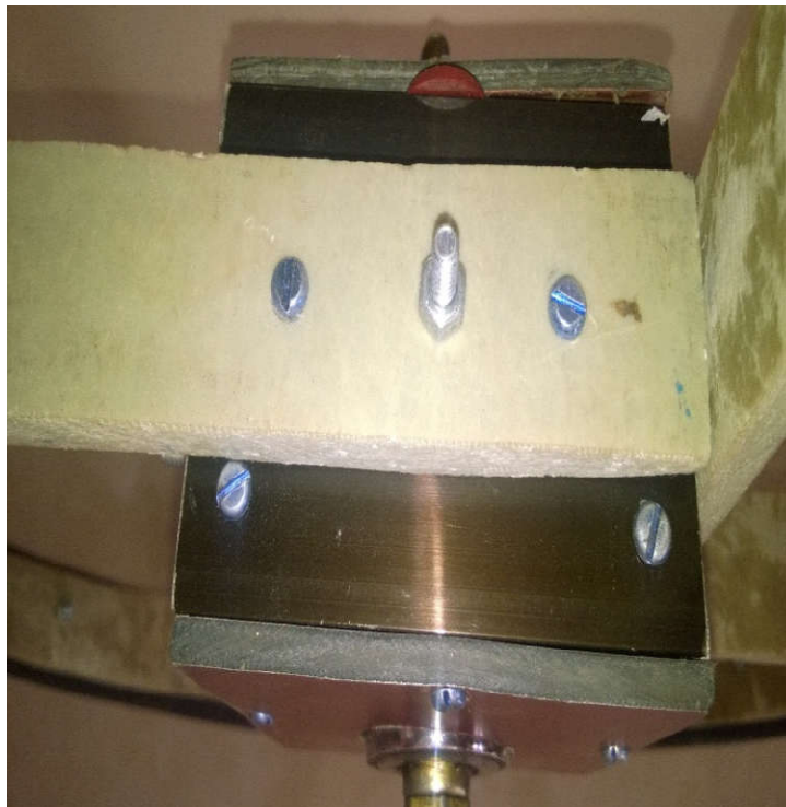
Fig. 11. Leaf Spring Fastening to Hub End.
