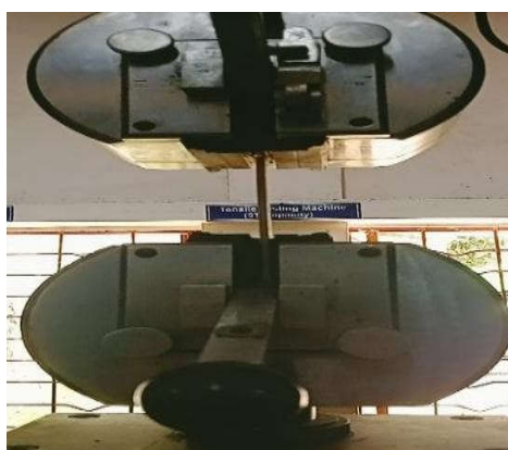
Fig.4. Tenso meter arrangement
