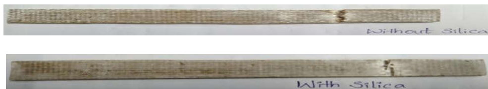
Fig.1.3 Tensile Specimen after Testing
