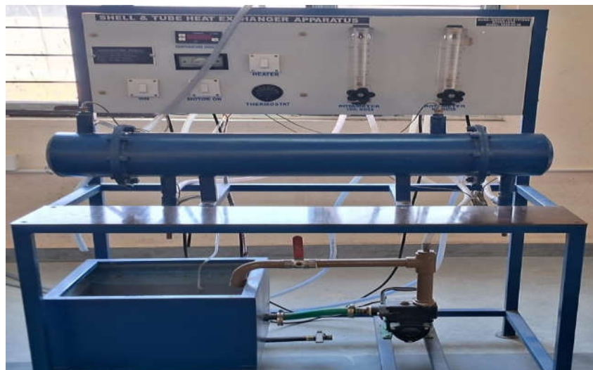
Fig 4: Experimental Setup of Shell and Tube Heat Exchanger
