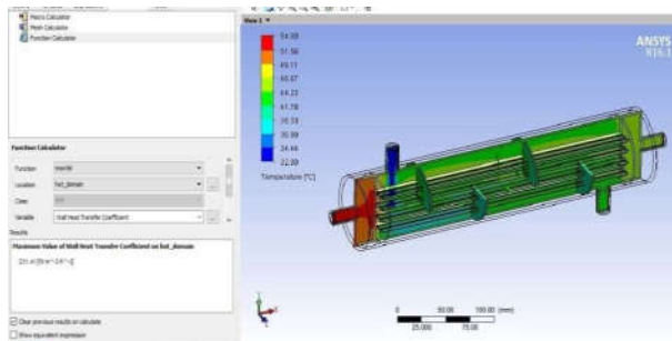
Fig 19: Maximum Value of Wall Heat Transfer Coefficient on Hot domain
