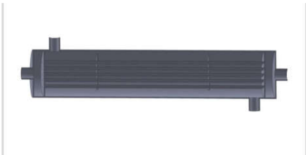
Fig 6: Heat Exchanger with 2 baffles
