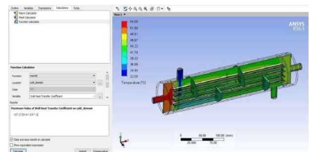
Fig 20: Maximum Value of Wall Heat Transfer Coefficient on Cold domain
