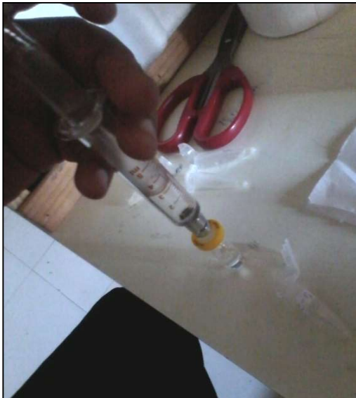
Plate 5: Filtration through 0.2 \mu m PTFE membrane filter in a vial.
