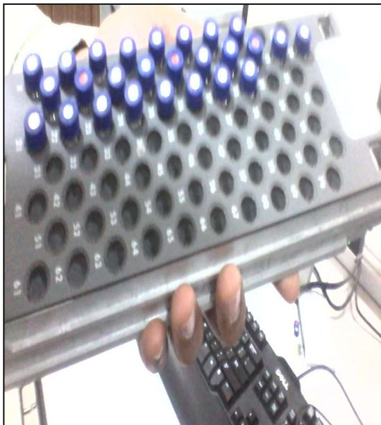
Plate 7: Vials are placed in a tray Plate 8: Setting of LCMS parameters.
